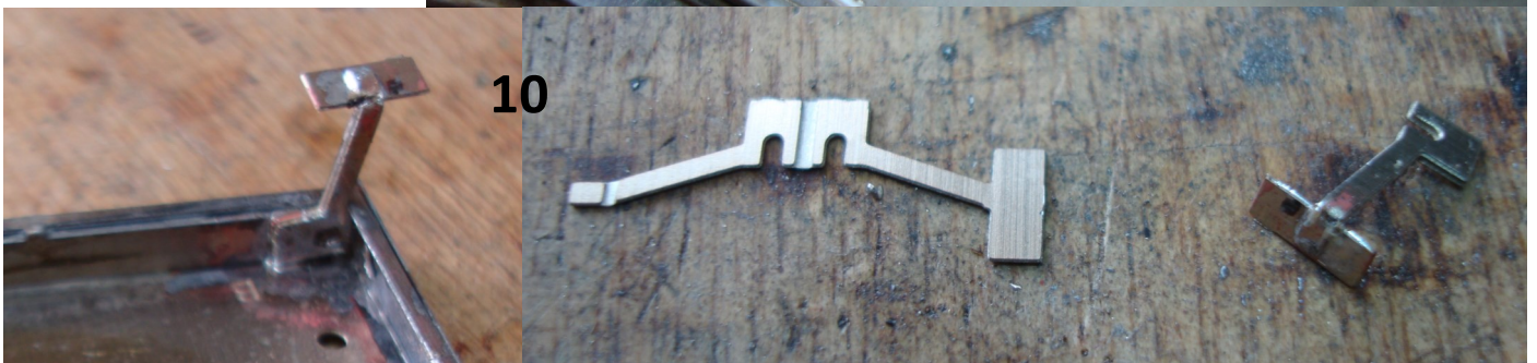
Completed underframes showing regulator box support platform in place.
